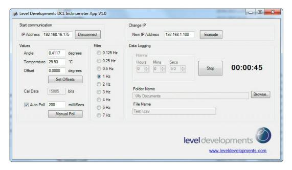
The device is shipped by default with the static IP address of 192.168.16.130. It should only be connected to a network where this address is free or reserved. After connection to the network and powering up the device, click the 'Connect' button to open the TCP/IP socket to the device. The angle and temperature values can then be retrieved by clicking the 'Poll' button. Checking the 'Auto Poll' check box will poll the device at regular intervals as specified in the relevant text
