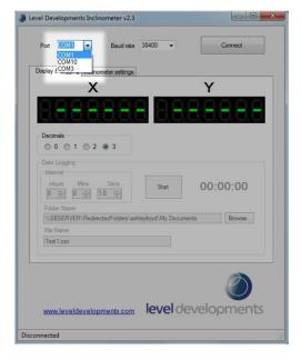
Run the Inclinometer App and select the port number that was determined earlier in Step 2.
