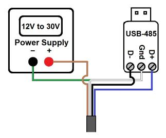
Once you've made all of the necessary connections you can switch on the power source or connect Pin 1 (brown) wire to "+" if using a battery.
