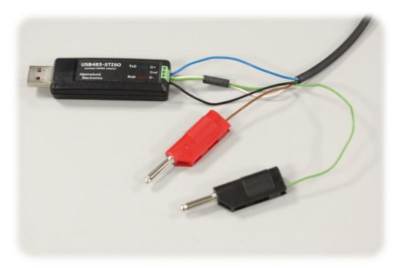
Note the additional green wire connected to the Gnd terminal to allow HPS Pin 2 to connect to -Ve power.
