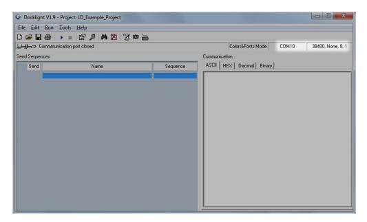
You can then change the COM channel (port number) to match the value determined in step 2.
