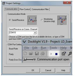
The default baud setting for all HPS sensors is 38400, with 8 data bits, 1 stop bit and no parity.
