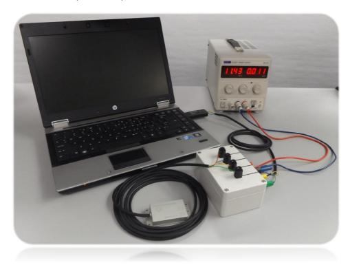
Once you've made all of the necessary connections you can switch on the power source or connect the red wire to "+" if using a battery.
