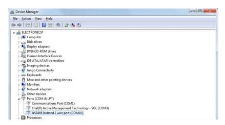
The name & port number that's automatically allocated to the USB to RS485 device can vary. Make a note of the port number that the device is allocated. Our example device is using "COM10" so this is the port number we would use to communicate with the inclinometer.
