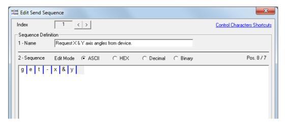
Send the new command to Inclinometer by clicking on the "—>" button.
