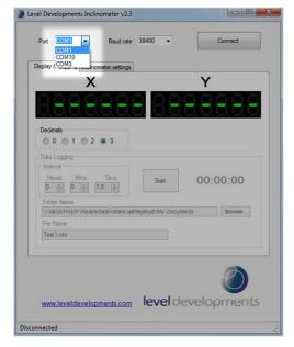
Run the Inclinometer App and select the port number that was determined earlier in Step 2.
