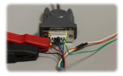
Back side of the female DB-9 connector & the required connections for RS232 communication. Note also that pin 5 of the DB-9 has 2 green wires fitted to allow connection to the Voltmeters.
