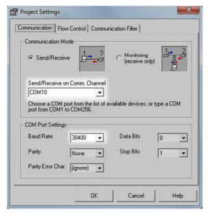
The default baud setting for all VS sensors is 38400, with 8 data bits, 1 stop bit and no parity.
