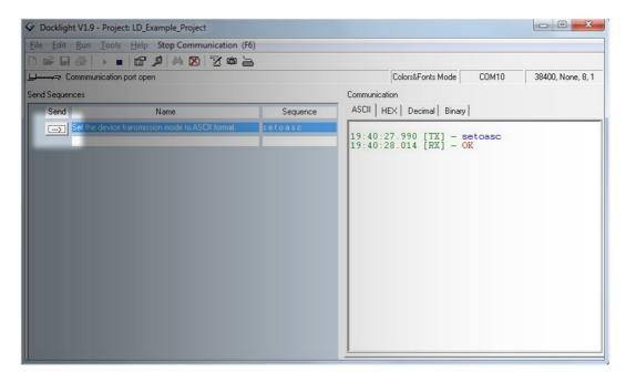
You can now create a 2nd command to request the angles from the Inclinometer.
