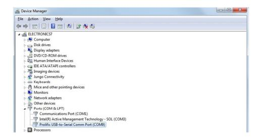
The name & port number that's automatically allocated to this device can vary. **Make a note of the port number that the device has been allocated**. Our example USB to COM device is using "COM9" so this is the port number we would use to communicate with the inclinometer.
