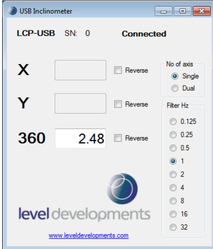
The USB interface is a HID model( Human Interface Device), and thus does not require a custom device driver to be loaded.
