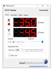
The device is supplied with a Free Windows based configuration application that can used to setup the display and trip angle. The display connects with a USB interface. It uses a the standard HID USB protocol so there is no need for any additional drivers as it utilises the standard Windows plug and play HID drivers. If another power supply is not connected to the device then the attached sensor will be powered from the USB port
